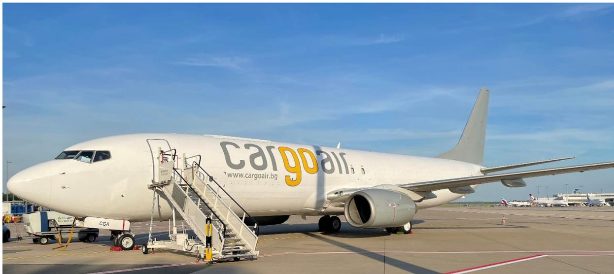
The AEI converted B737-800SF freighter offers a main deck payload of up to 52,700 lbs. (23,904 kg) and incorporates eleven full height 88" x 125" container positions, plus an additional position
